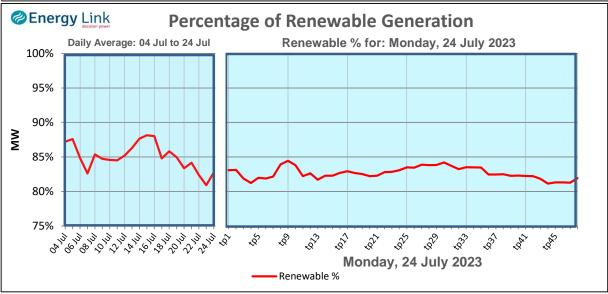
Note: For the purposes of this chart, renewable generation is all hydro, geothermal, wind and grid scale solar. Co-generation is counted as thermal generation even though the carbon may be attributed to other industries.
