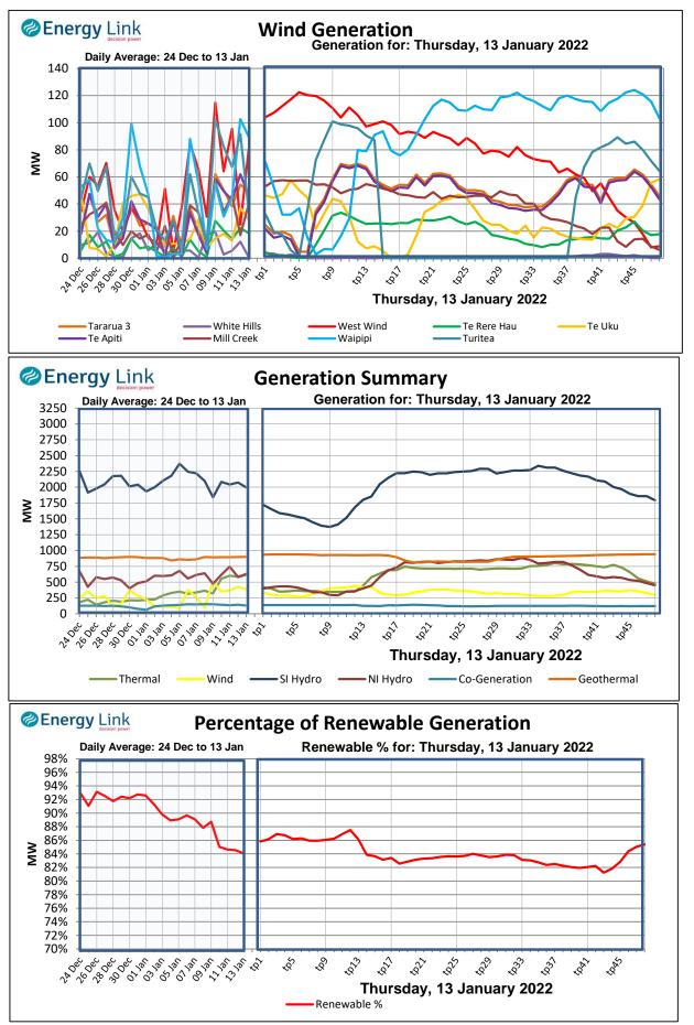
Note: For the purposes of this chart, renewable generation is all hydro, geothermal, wind and grid scale solar. Co-generation is counted as thermal generation even though the carbon may be attributed to other industries.
